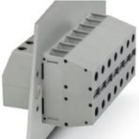
Panel feed-through terminal block, connection method: Screw connection with tension sleeve, Screw connection with tension sleeve, number of positions: 1, load current: 101 A, cross section: 6 mm<sup>2</sup> - 35 mm<sup>2</sup>, width: 15.1 mm, color: gray
