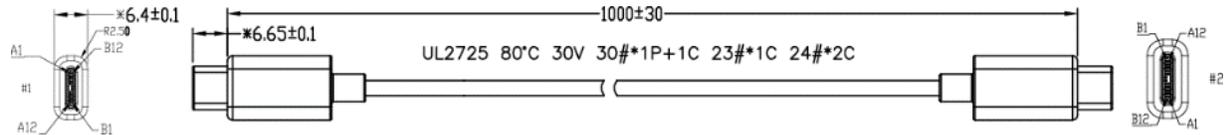
UES-1003A160: Low Drop Type-C USB Cable – 1 Meter – 23AWG on Power – 30AWG on Data – Black (mm)
