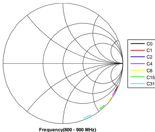
Figure 6. Measured Step Size vs State (frequency)
