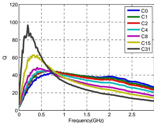
Figure 9. Measured Shunt Q vs State
