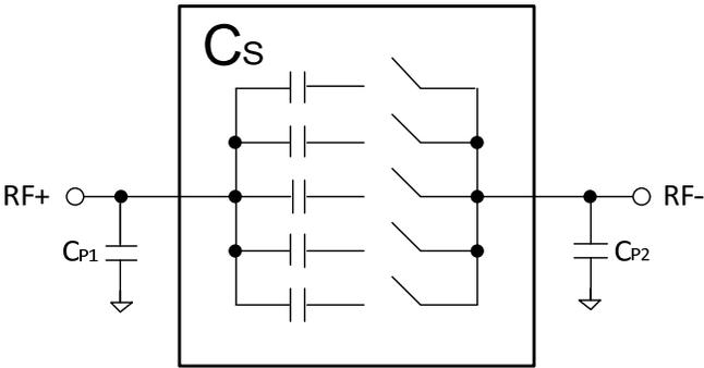
Shunt Configuration (looking into RF+ when RF- is grounded) will have higher total capacitance at RF+ due to parallel combination of  $C_s$  with parasitic capacitance  $C_{P1}$  ( $C_s + C_{P1}$ ), as demonstrated in Figure 14 and Table 9.
