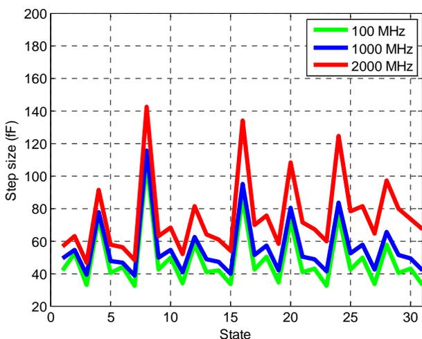
Figure 7. Measured Shunt C vs Frequency (major states)
