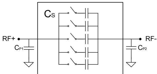
Shunt configuration (looking into RF+ when RF- is grounded) will have higher total capacitance at RF+ due to parallel combination of  $C_S$  with parasitic capacitance  $C_{P1}$  ( $C_S + C_{P1}$ ), as demonstrated in Figure 15 and Table 9.
