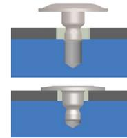
The Belleville shaped head flattens upon a simple press-in installation and draws panels together to accommodate vertical stack tolerances.
