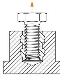
**Pullout** is the force required to pull the insert from the sheet.
