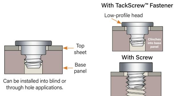
Typical screw related issues include costly tapping, cross-threading, torque control, and vibration back out
