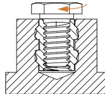
**Torque-out** is the torque required to turn the insert in the parent material after installation without inducing clamp load on the fastener.
