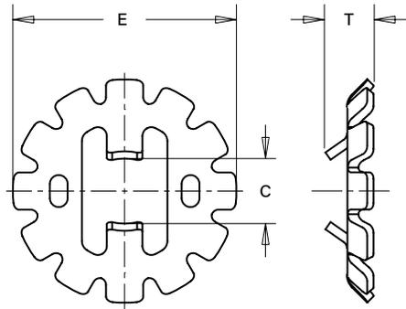
The ClampDisk® fastener can be used with a self-clinching pin. Contact [techsupport@pemnet.com](mailto:techsupport@pemnet.com) for information on pin material options.
