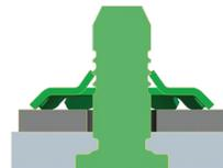
The PEM® ClampDisk® fastener can be installed onto a grooved pin for increase strength and allow installation onto any material. For more information, contact [techsupport@pemnet.com](mailto:techsupport@pemnet.com).
