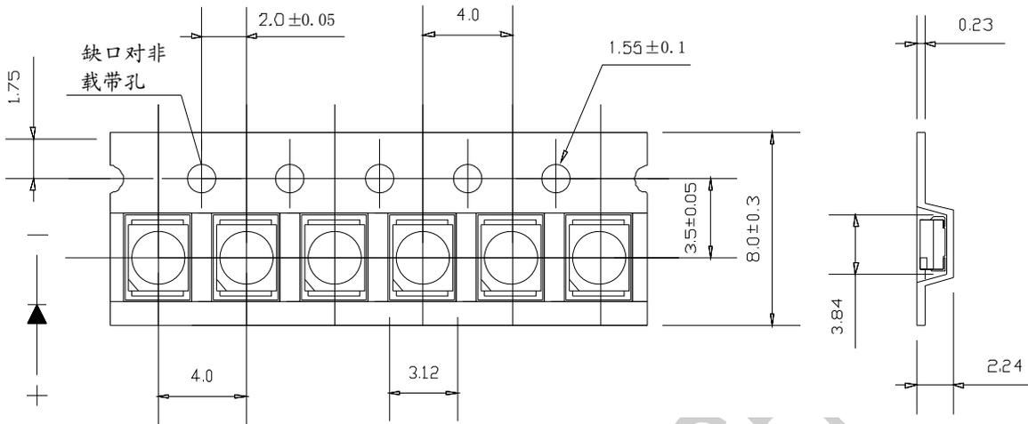
Note: Tolerance unless mentioned is  $\pm 0.1$ mm; Unit = mm
