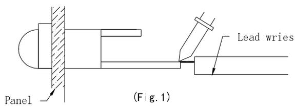
2) When soldering wire to the lead, work with a Fig (See Fig.2) to avoid stressing the package.
