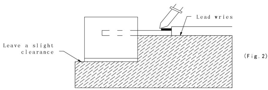
Regarding solution in the tinning oven for product-tinning, compound sub-solution made of tin & copper and silver is proposed with the temperature of Celsius 260. The proportion of the alloyed solution is tin 95.5: copper 3.5: silver 0.5 by percentage. The time of tinning is constantly 3 seconds.
