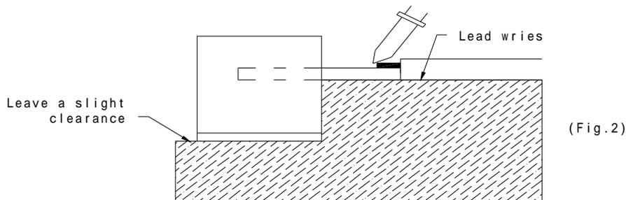
Regarding tinning the leads, compound made of tin, copper and silver is proposed with the temperature of 260°C. The proportion of the alloyed solution is 95.5% tin, 3.5% copper, 0.5% silver. The time of tinning is 3 seconds.
