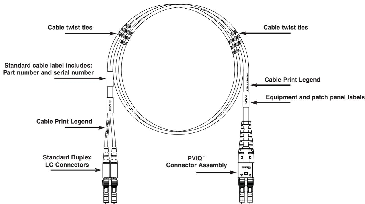
**Example Description: PVQ9PE10LQM05.0** = PanView™ Interconnect Fiber Patch Cord, 9/125µm singlemode, OFNP 1.6mm jacketed, standard duplex LC – to – PanView™ Duplex LC, 5.0 meters long
