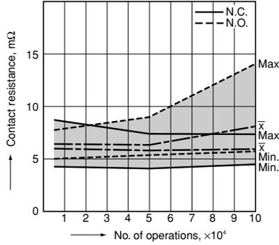
3. Electrical life (SP4, 10 A 250 V AC resistive load)
