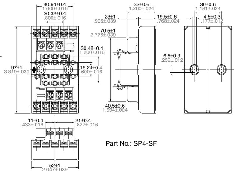
Note: Terminal number marking is on the socket body. Please refer together with the SP relay schematic.
