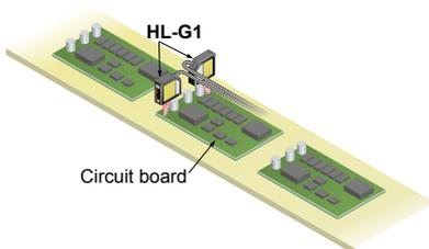
**Measurement of sheet thickness**
