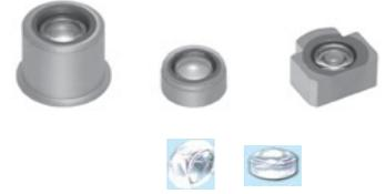
These products are aspherical glass lenses by using a press molding, and key devices of optical electronics not only provide compact and light weight but also high-performance by utilizing characteristics of aspherical design.
