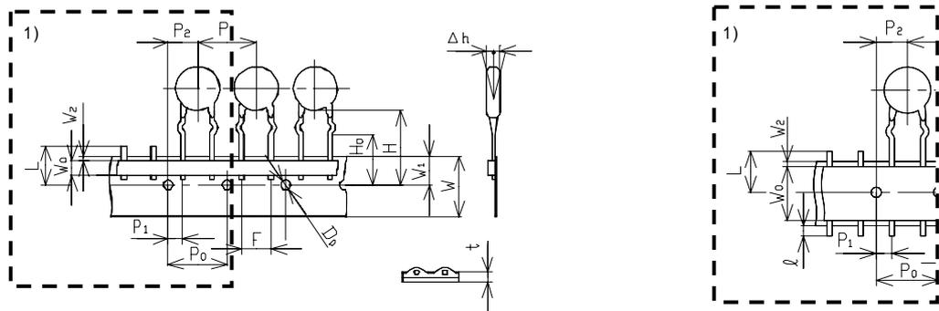
Fig. 1.4 Crimped Leads and Taping
