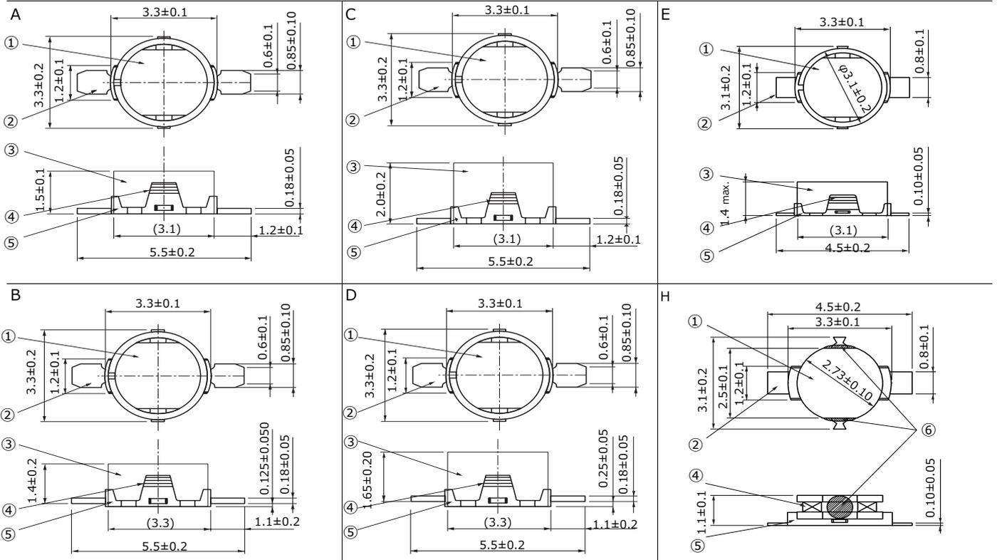
Part Name: ①Core ②Terminal ③Ring ④Coil ⑤Terminal board ⑥Adhesive
