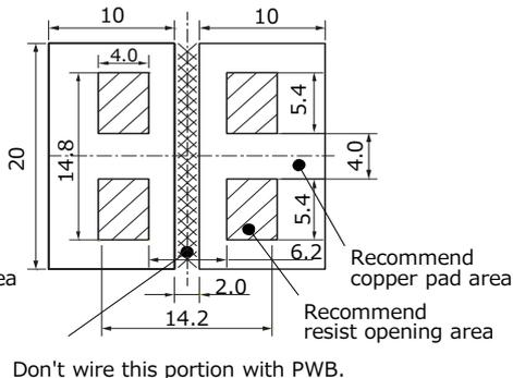
**■ As for Soldering Conditions and Safety Precautions (Power Choke Coils (Automotive Grade)),**
