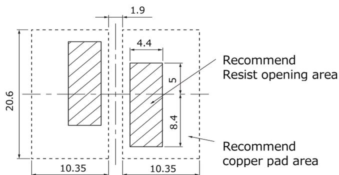
\* Due to bigger part, Thermal Capacity is large and may occur PWB temperature differences during reflow process. Recommended land pattern (Heat absorb) should be designed with reflow mountability.
