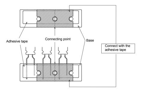
Note ) When connecting two base tapes, they shall not be piled on top of each other. Base tapes shall not be connected with each other by using staples.
