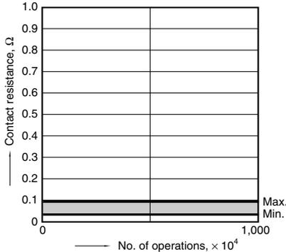
2-(2). Change in dynamic contact resistance (10 μA 1 mV DC resistive load)
