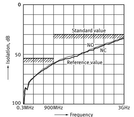
1-4.High frequency characteristics (75 Ω, Surface mount terminal)
