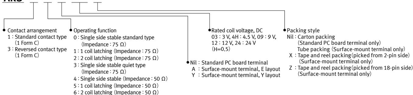
Note : Packing style symbol "X", "Z" is not marked on the relay.
