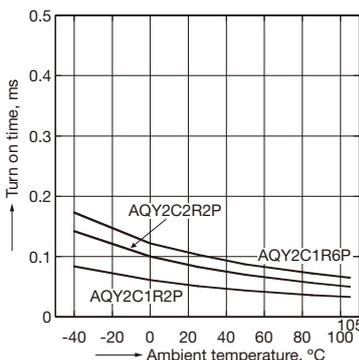
3-(2). Turn on time vs. ambient temperature characteristics
