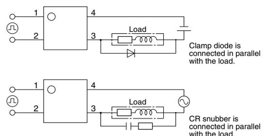
2) When Clamp diode or CR Snubber is used in the circuit, the spike voltages from the load are limited. But the longer wire may become the inductance and cause the spike voltage. Keep the wire as short as possible.
