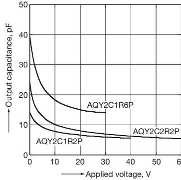
13-(2). Output capacitance vs. applied voltage characteristics
