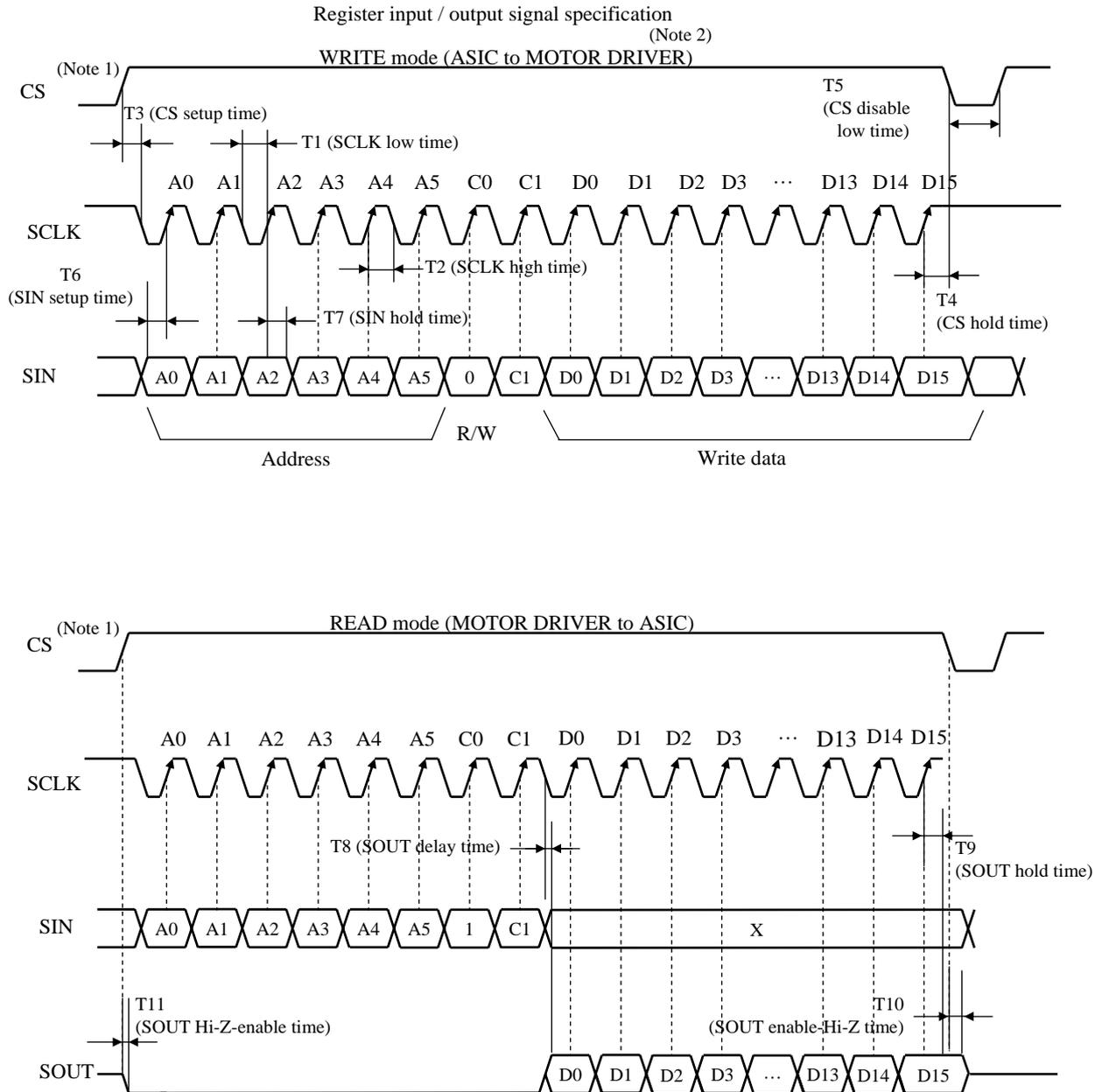
Note 1) CS default value of each cycle (Write / Read mode) starts from Low-level.
