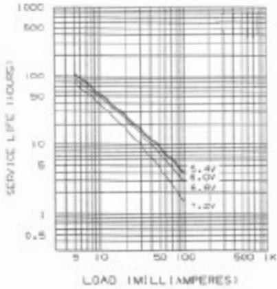
**Typical Discharge Characteristics with Constant Resistance at 20°C**
