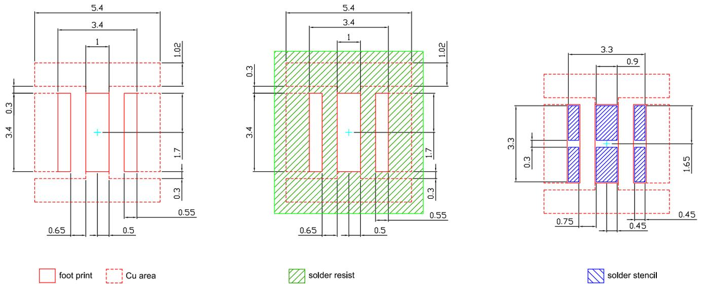
For superior solder joint connectivity results we recommend soldering under standard nitrogen atmosphere. Further information can be found in our Application Note: "Handling and Processing Details for Ceramic LEDs". Package not suitable for any kind of wet cleaning or ultrasonic cleaning.
