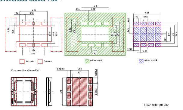
For superior solder joint connectivity results we recommend soldering under standard nitrogen atmosphere. Package not suitable for any kind of wet cleaning or ultrasonic cleaning.
