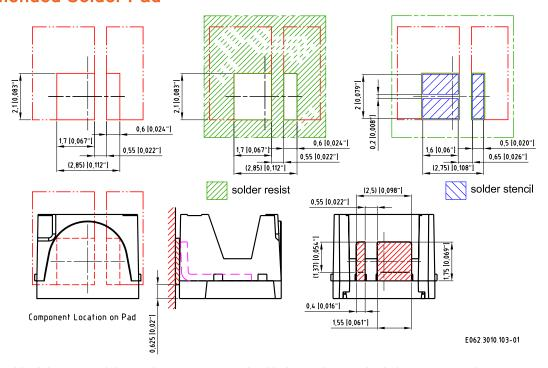
For superior solder joint connectivity results we recommend soldering under standard nitrogen atmosphere.
