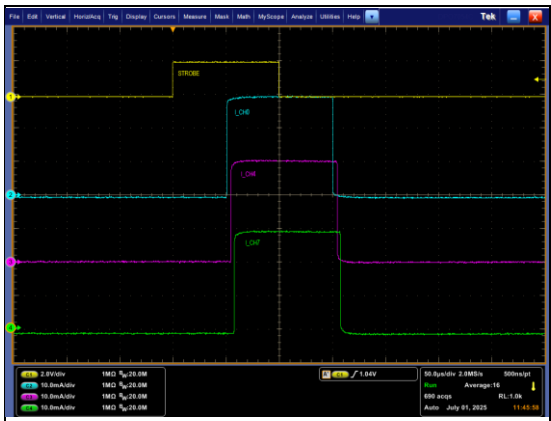
Figure 5: 1 PWM input, T_STAGGER = 1µs
