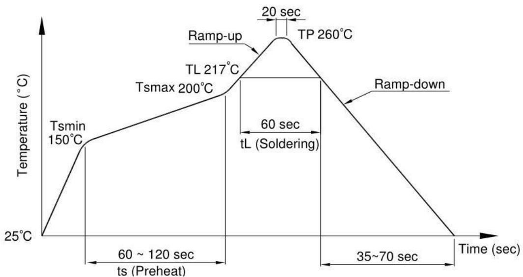
**(3) .Wave soldering (JEDEC22A111 compliant)**
