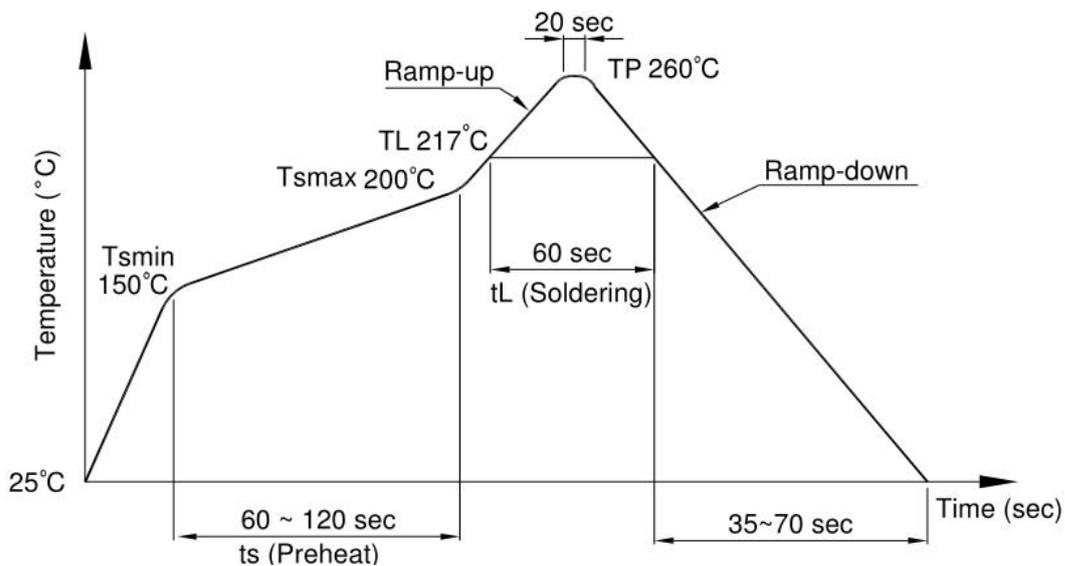
(2) Wave soldering (JEDEC22A111 compliant)
