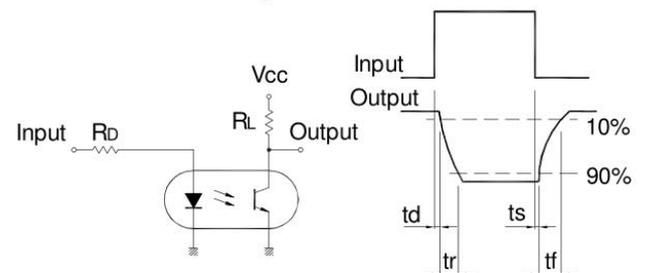
Test Circuit for Frequency Response
