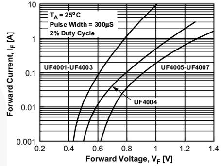
Figure 2. Forward Characteristics
