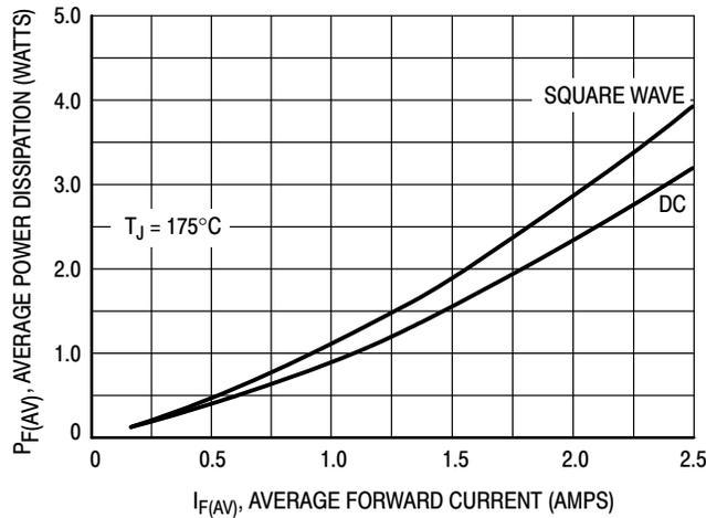
**Figure 7. Power Dissipation**
