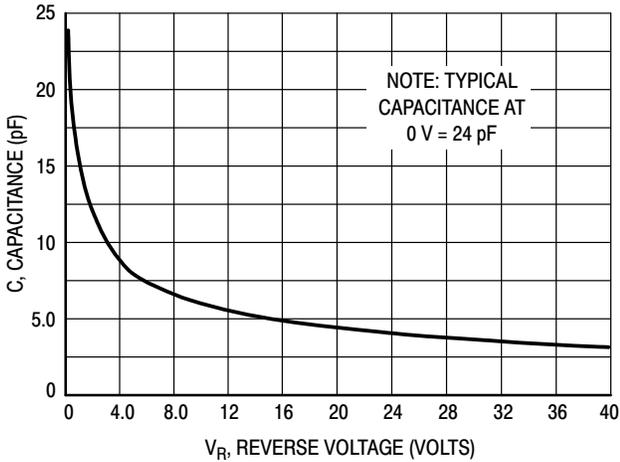
**Figure 5. Typical Capacitance**
