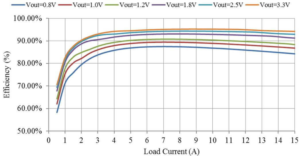
Figure 16. Efficiency vs. Load Current (Vin=12 V)
