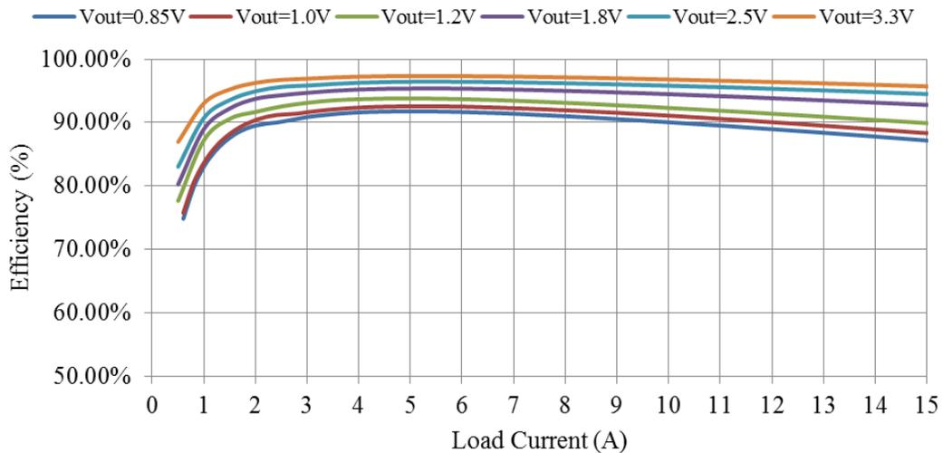
Figure 17. Efficiency vs. Load Current (Vin=5.5 V)
