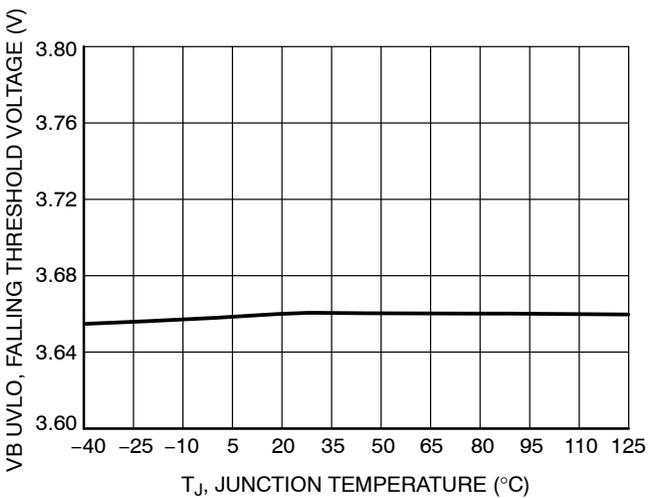
Figure 13. VB UVLO Falling Threshold vs. Junction Temperature
