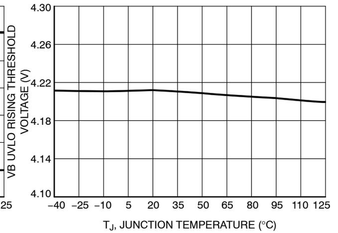
Figure 12. VB UVLO Rising Threshold vs. Junction Temperature
