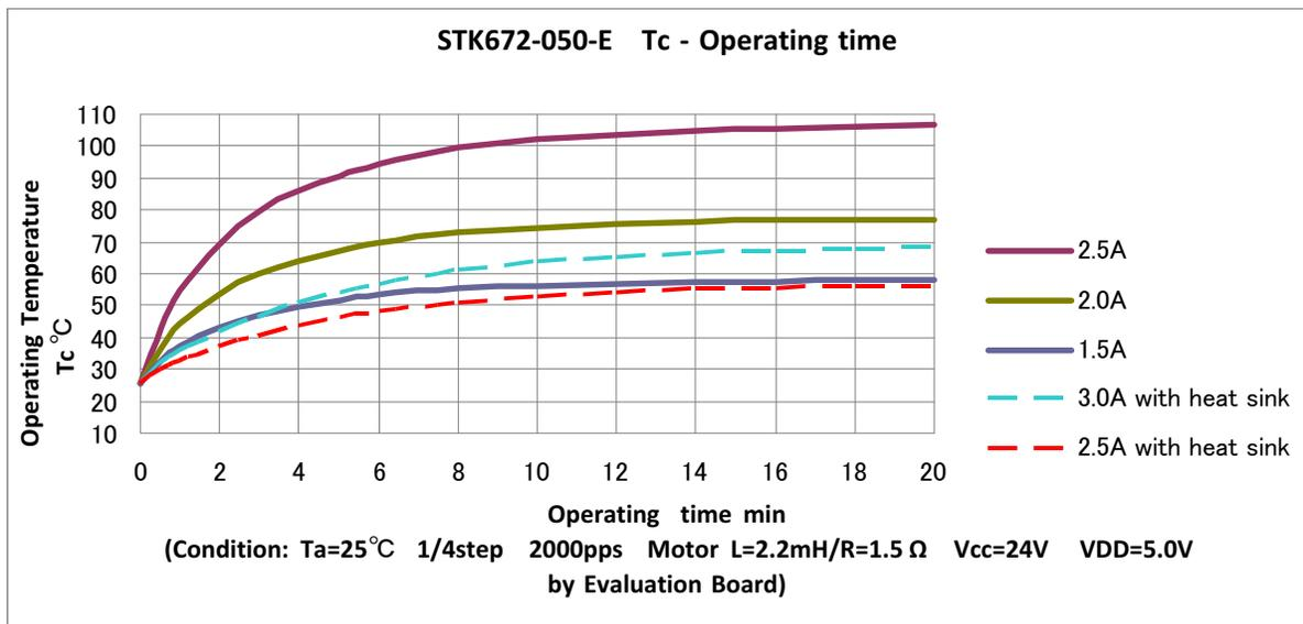
Figure 7. Operating Temperature
