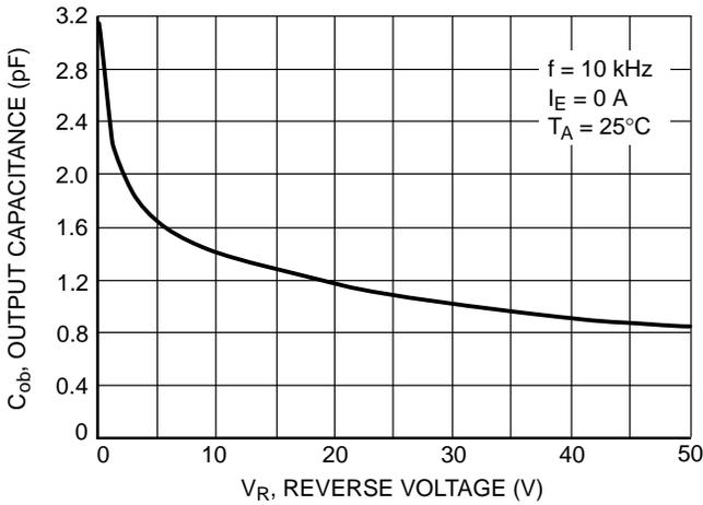
Figure 4. Output Capacitance
