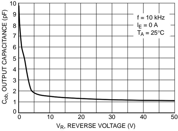
Figure 9. Output Capacitance
