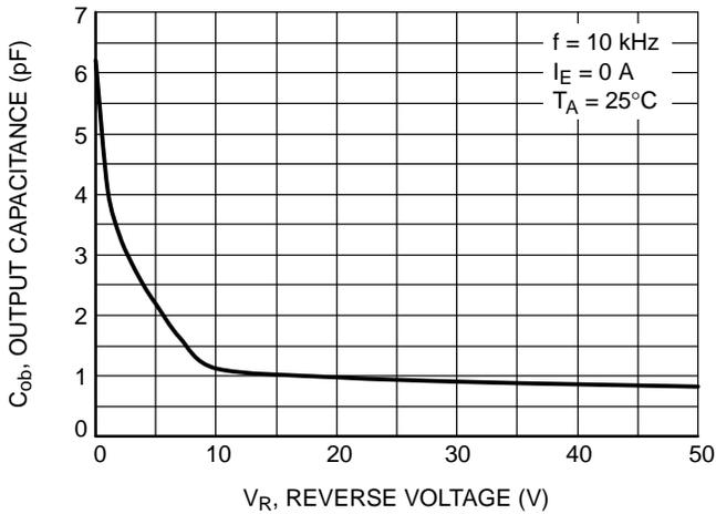
Figure 19. Output Capacitance
