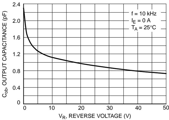
Figure 14. Output Capacitance
