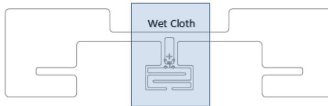
**Figure 1. Moisture Contact Test Area**
