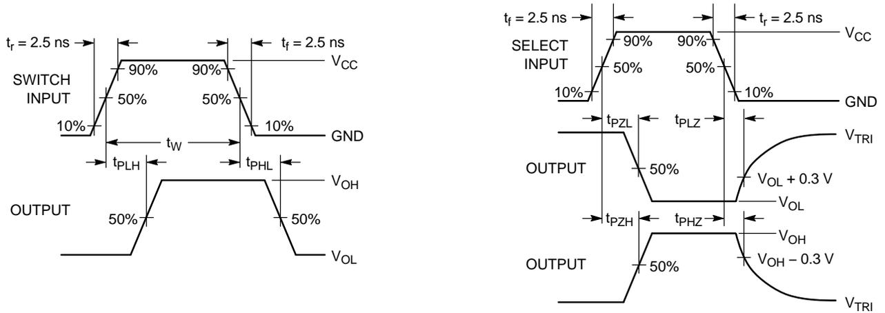
Figure 3. AC Waveforms
