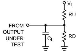
Figure 2. AC Test Circuit
