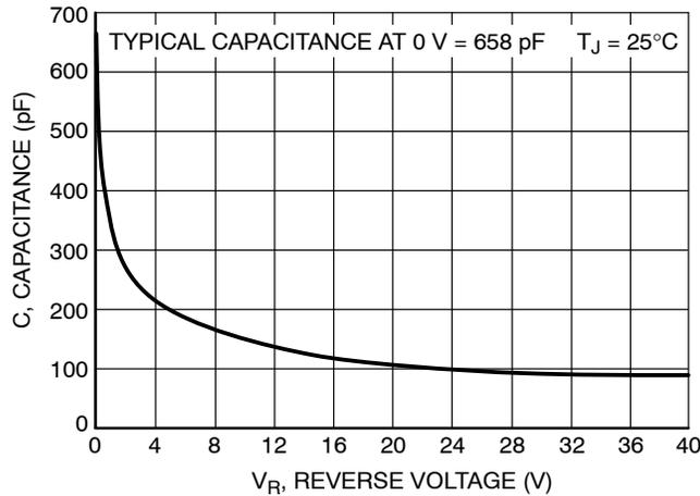
**Figure 7. Typical Capacitance**
