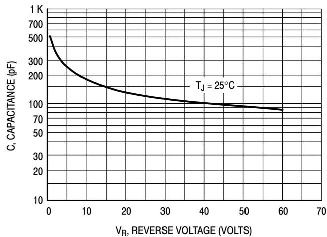
Figure 6. Typical Capacitance
