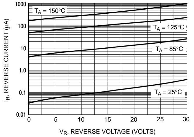
Figure 3. Leakage Current
