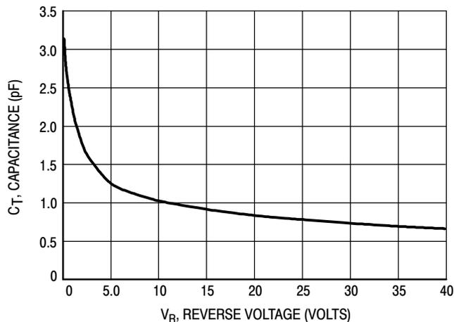
Figure 3. Typical Capacitance
