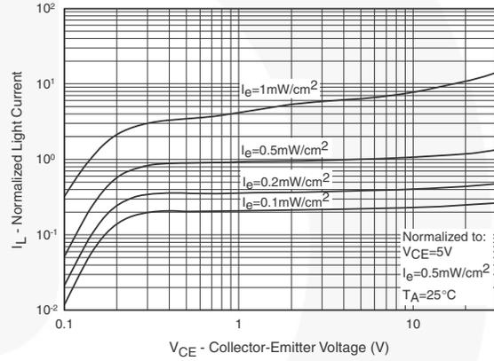
**Figure 4. Light Current vs. Collector - Emitter Voltage**
