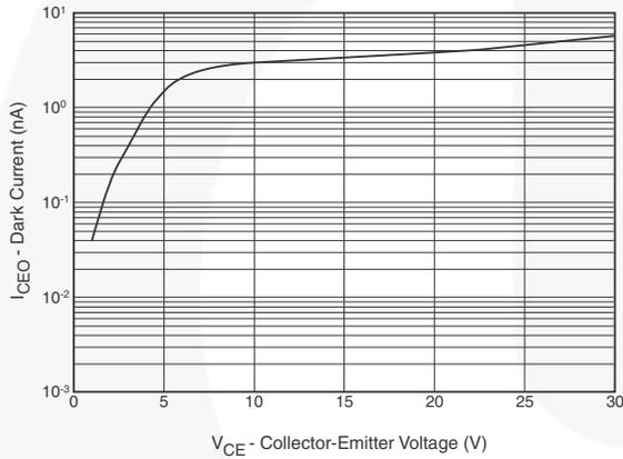
**Figure 3. Dark Current vs. Collector - Emitter Voltage**
