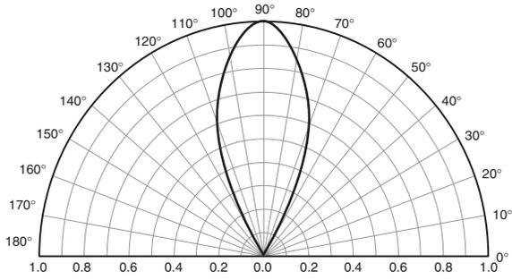
**Figure 8. Coupling Characteristics of QED22X and QSD22X**
