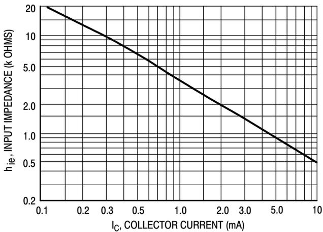
Figure 13. Input Impedance
