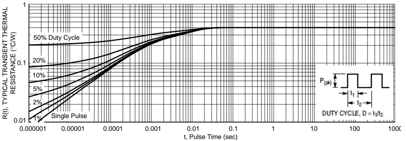
Figure 9. Typical Transient Thermal Response, Junction-to-Case for NTSB30100CTG
