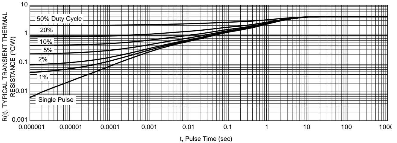
Figure 8. Typical Transient Thermal Response, Junction-to-Case for NTSJ30100CTG
