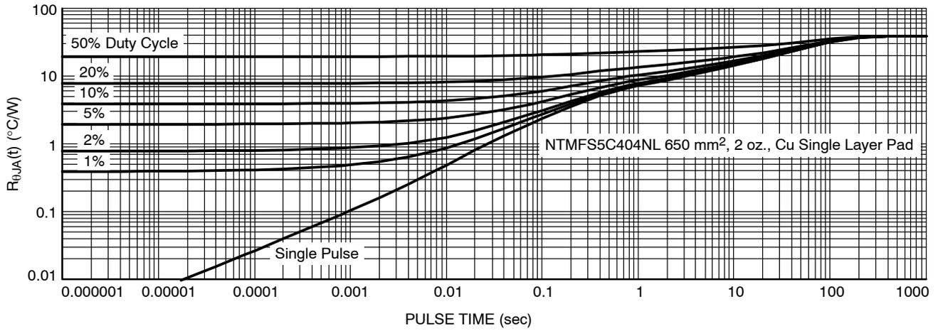
Figure 13. Thermal Characteristics
