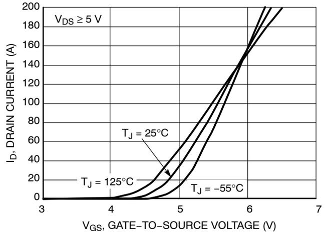
Figure 2. Transfer Characteristics
