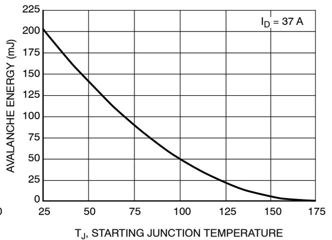
Figure 12. Maximum Avalanche Energy versus Starting Junction Temperature
