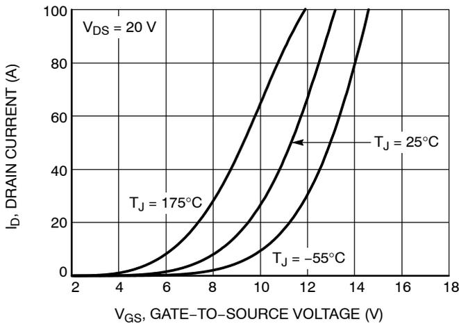
Figure 5. Transfer Characteristics
