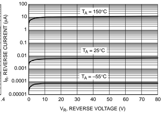
Figure 3. Reverse Leakage
