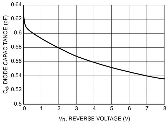
Figure 4. Diode Capacitance
