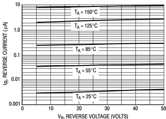
Figure 3. Leakage Current
