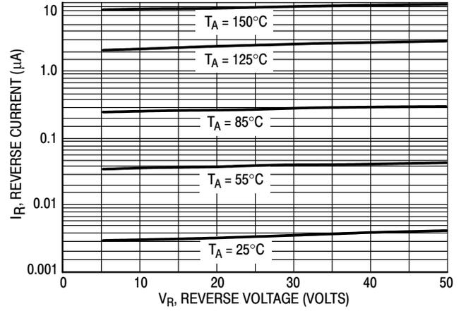
Figure 3. Leakage Current
