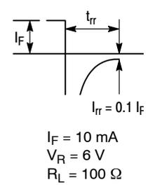
Figure 1. Reverse Recovery Time Equivalent Test Circuit
