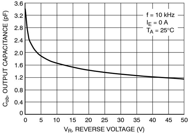
Figure 4. Output Capacitance
