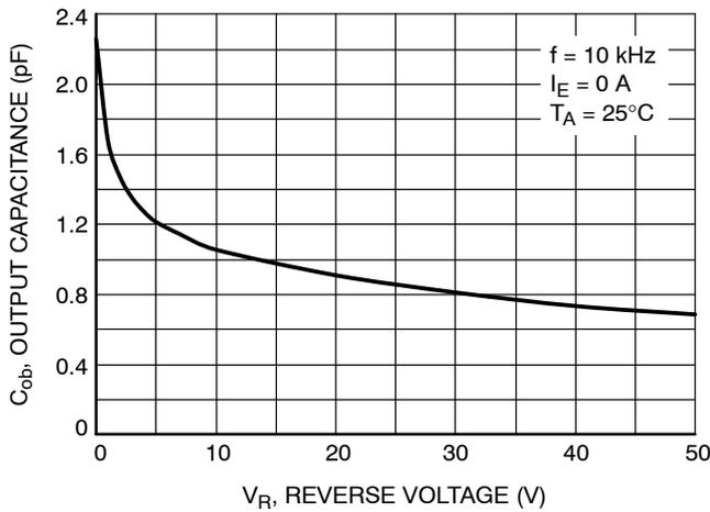
Figure 9. Output Capacitance
