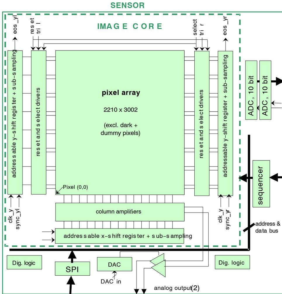
Figure 4. Floor Plan
