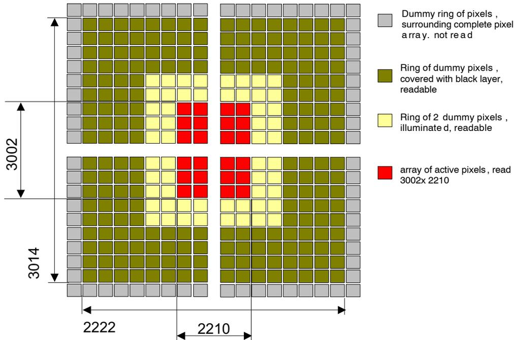
**Figure 6. Floor Plan Pixel Array**
