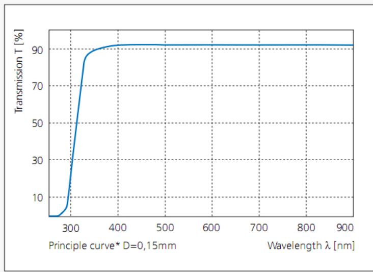
**Figure 23. Transmission Characteristics of the Glass Lid**
