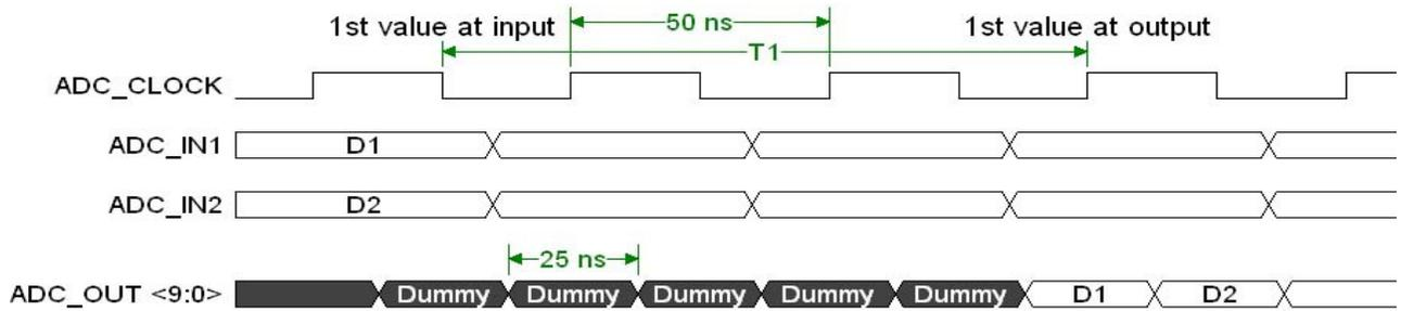
**Figure 21. ADC Timing using Two Analog Outputs**
