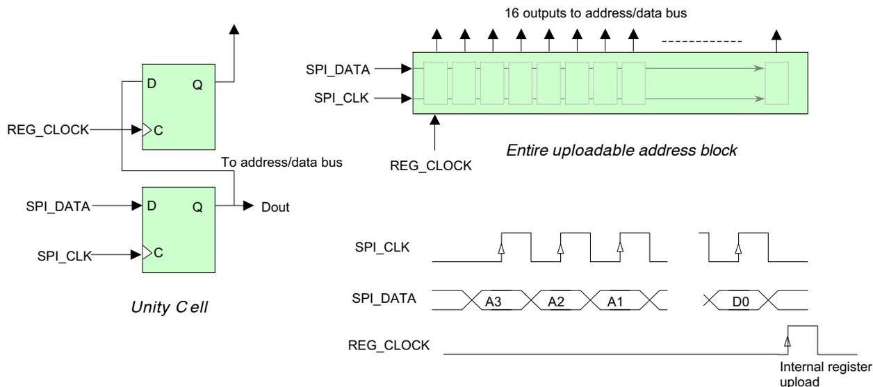
**Figure 9. SPI Interface**
