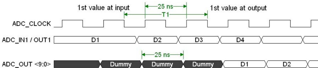
**Figure 22. ADC Timing using One Analog Output**
