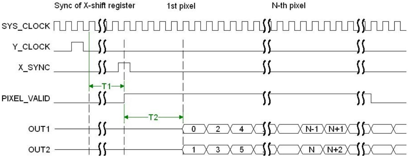
**Figure 19. Pixel Output Timing using Two Analog Outputs**
