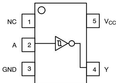
Figure 1. Pinout
